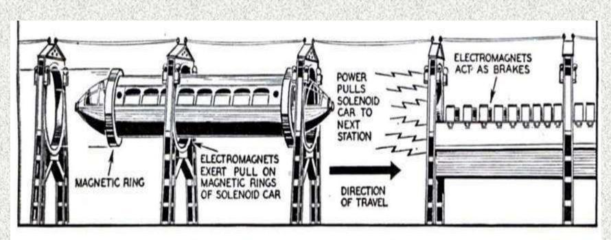
The artist's drawing at top illustrates the solenoid rapid transit railway now being developed by German engineers. Cars speed forward under power of giant solenoids exerting powerful pull on magnetic rings around the cars. Current to next solenoid in line is switched on automatically when fast moving car intercepts light beam from photo electric cells. Diagram shows operation of solenoids.
