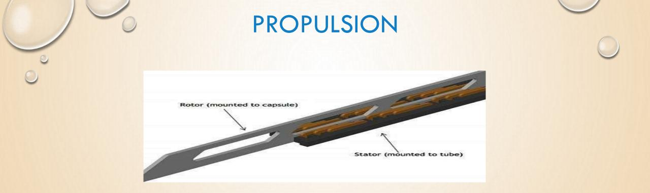
• LINEAR ACCELERATION ARE CONSTRUCTED ALONGTHE LENGTH OF THE TUBE AT VARIOUS LOCATION TO ACCELERATE THE CAPSULE ST ATACS ARE LOCATED ON THE CAPSULE VIA THE LINEANR ACCELERATION.
