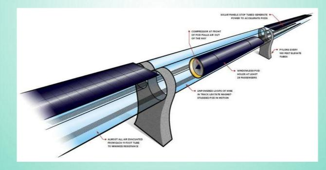
• IN THE CONSTRUCTION OF HYPERLOOP THE TUBE IS CONSTRUCTED ON THE CONCRETE PILLARS. THE DIFFERENCE BETWEEN TWO PILLARS IS 100 FEET.
